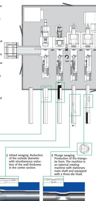
Expanding: Production of the pre-diameter for the internal spline on a hydraulic axial forming machine. <u>2</u> Infeed swaging: Production of the internal spline by swaging over a profiled mandrel.
