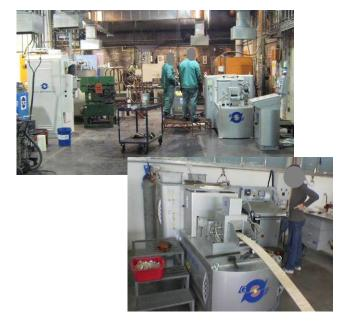
The horizontal continuous casting furnace **LOGIC**, with induction heating system, has been conceived to produce wires, plates, tubes and customized special sections.
