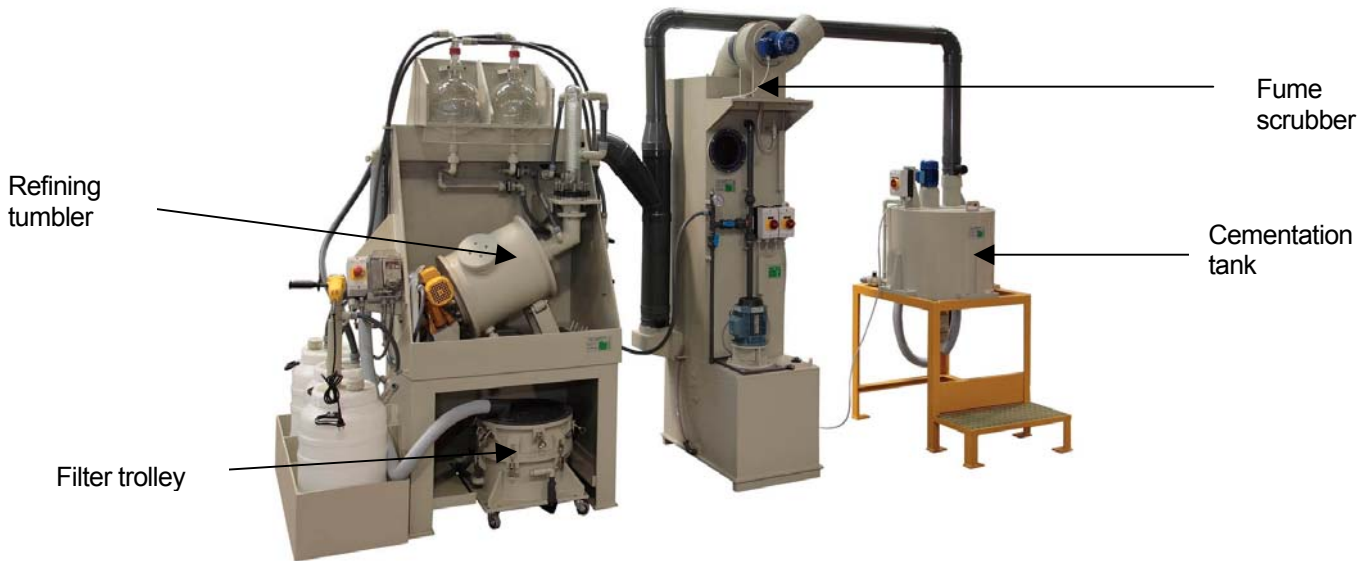
Fig. 6 - IAQ25BR refining plant and fume scrubber
